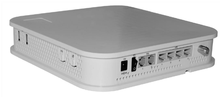
Figura 6: CISCO ONT ME4600 Residential Gateway User Manual Fuente: ME4600 Optical Network Termination Residential Gateway User Manual (CISCO SYSTEMS, INC., 2017)
